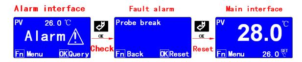
Note: After checking the fault, pls remove it first, then reset the chiller.
